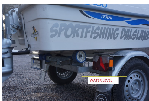
3. Mind the waterlevel, trailer lights are not waterproof
